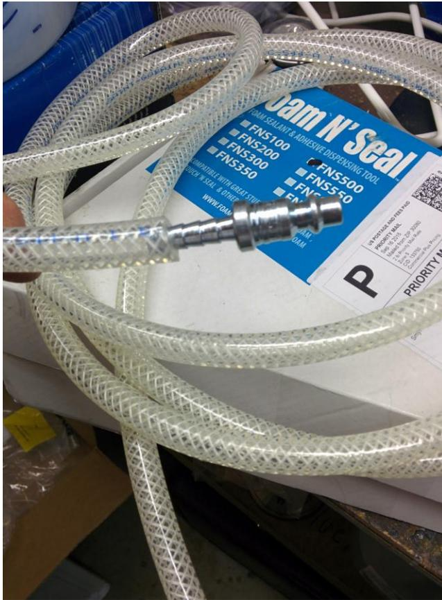
I bought this fitting to use on the above hose to adapt it to my compressed air fittings. McMaster.com p/n 6534K66.
